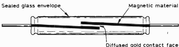
Fig. 4: Reed relay contacts.
